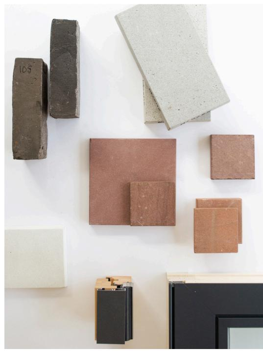
Range of materials including red sandstone and white precast concrete and black anodised aluminium
